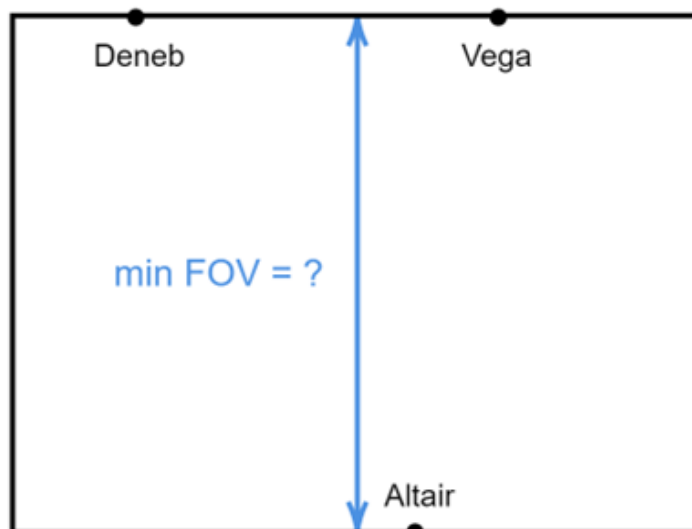
Figure 3: Astley's camera configuration for photographing the Summer Triangle.
